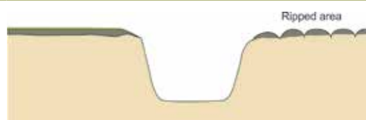
Rip gully edge prior to removal of topsoil
