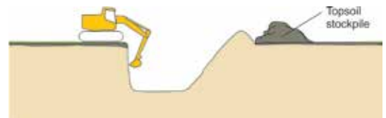
Shaping gully sides with excavator
