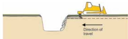
The rippers are lowered and the bulldozer reversed to gully edge, pushing soil down gully sides
