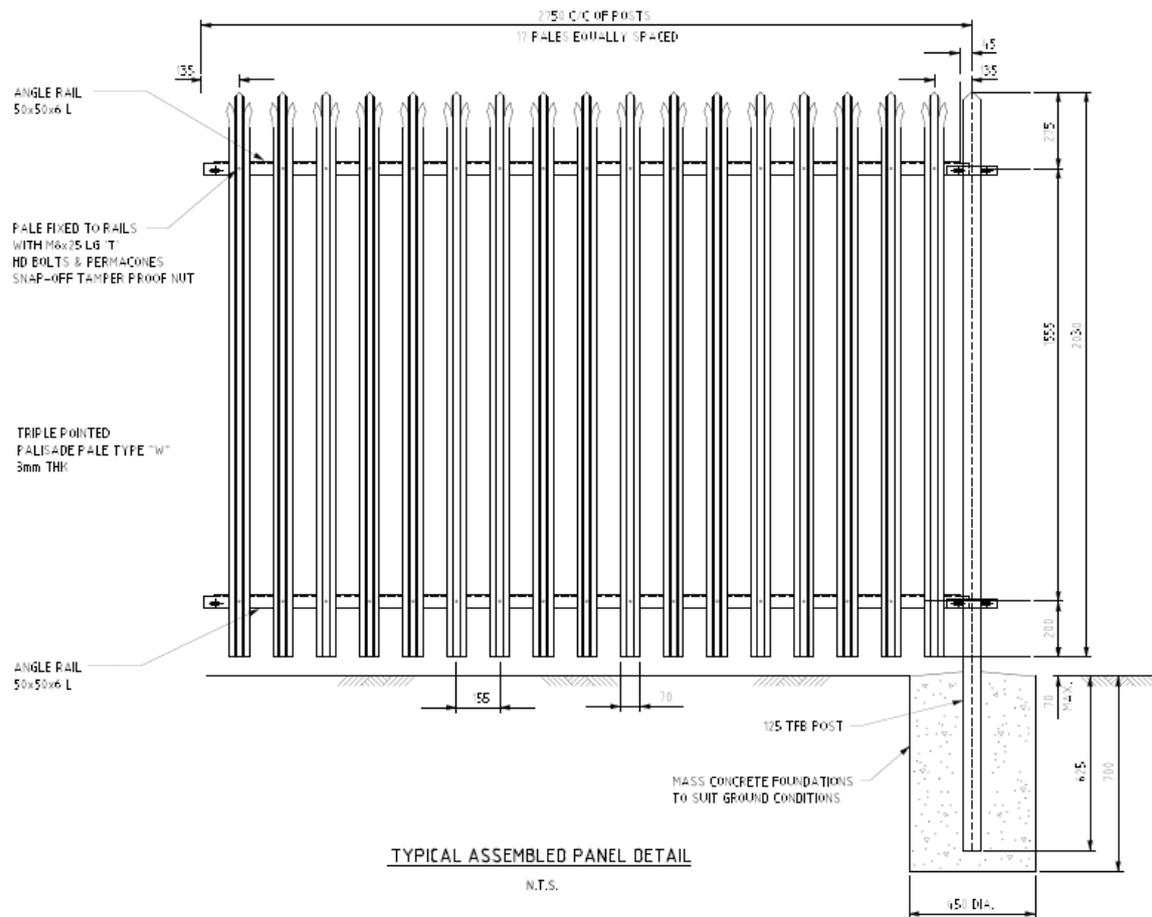
**Figure 15 - Palisade fence drawing (WaterNSW ref: PL2019/254)**
