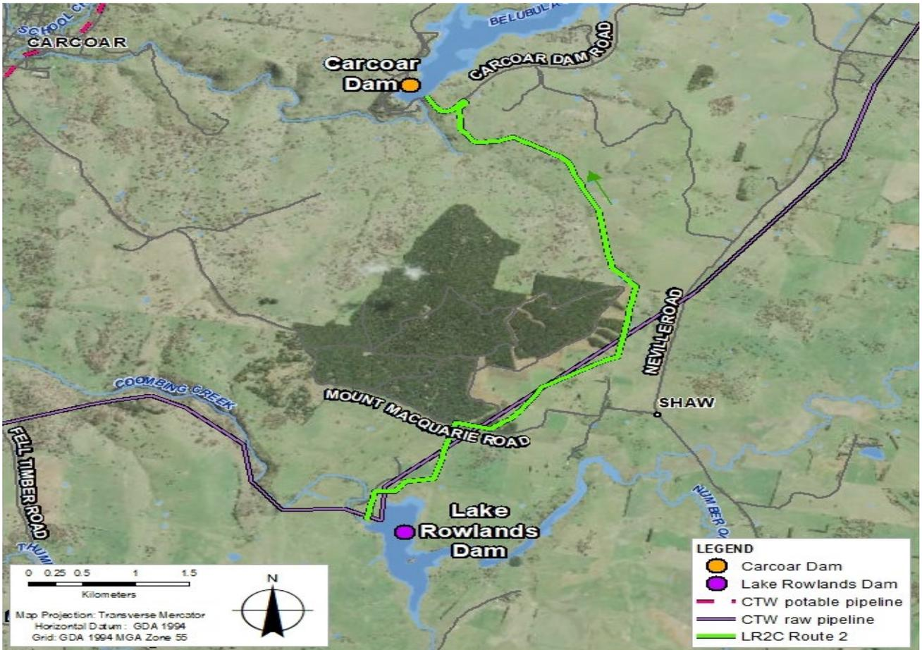
Proposed option – Lake Rowlands Dam to Carcoar Dam Pipeline alignment
