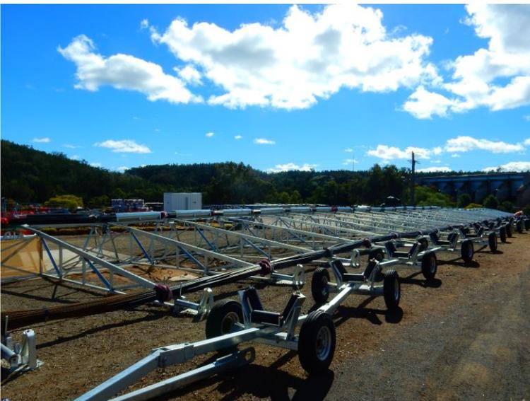
Trolleys designed for transporting the anchors
