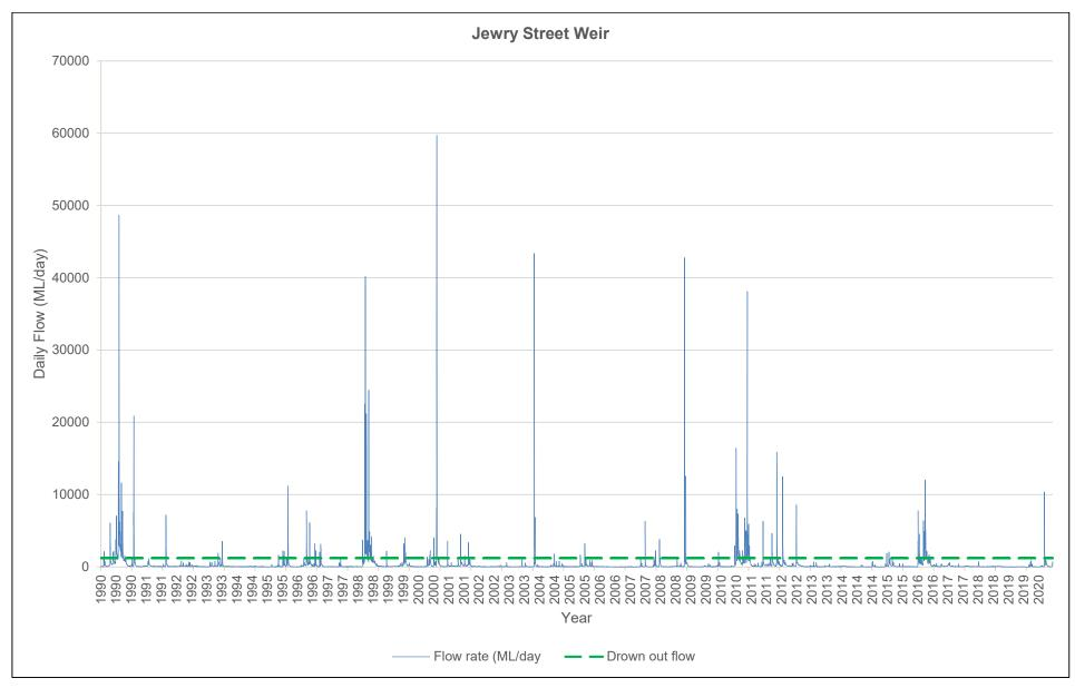
Figure 37. Fish passage availability at Jewry Street Weir over a 30 year period. Green line indicates approximate flow volume at which fish passage is possible
