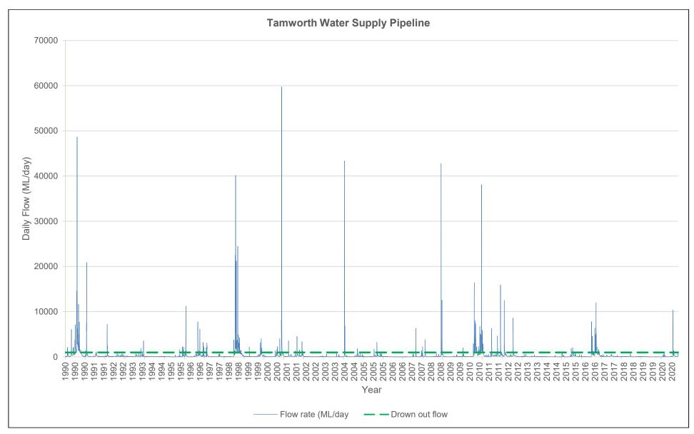
Figure 36. Fish passage availability at Tamworth Water Supply over a 30 year period. Green line indicates approximate flow volume at which fish passage is possible
