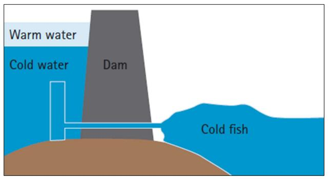
*Figure 41.* Cold water pollution occurs through drawing of water from the bottom of large storages (NSW DPI, 2005).
