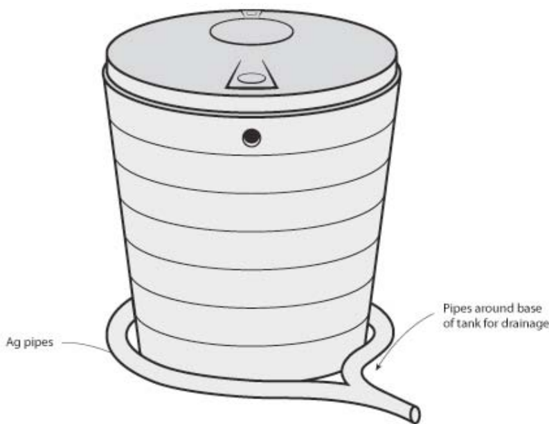
Figure 3.2 Ag pipes around base of septic tank for drainage
