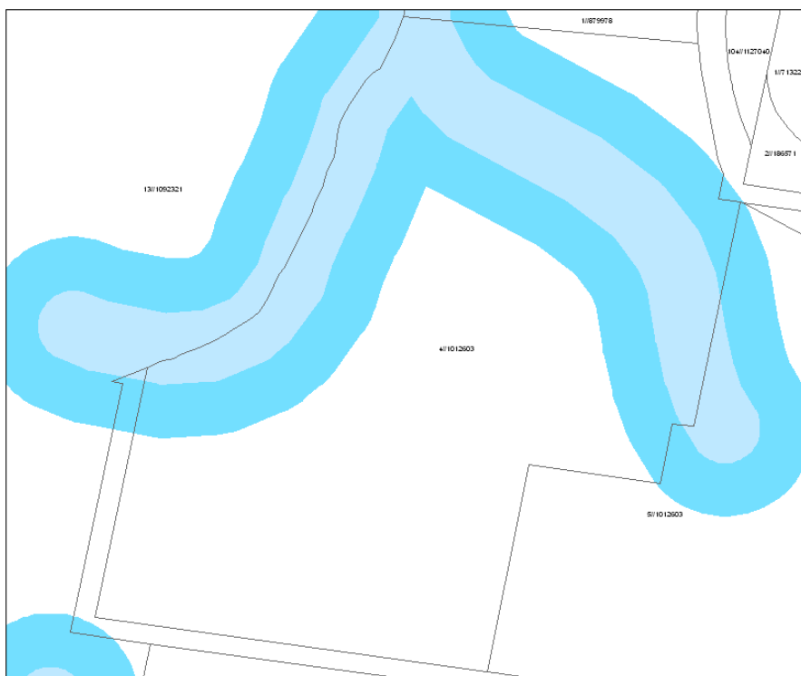
Figure 2-12 Watercourse constraint mapping for proposed subdivision – drainage depressions and farm dams need to be identified through a site inspection.
