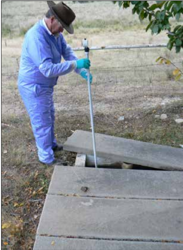
Figure 4.6 Testing sludge depth using a 'Sludge Depth Indicator'
