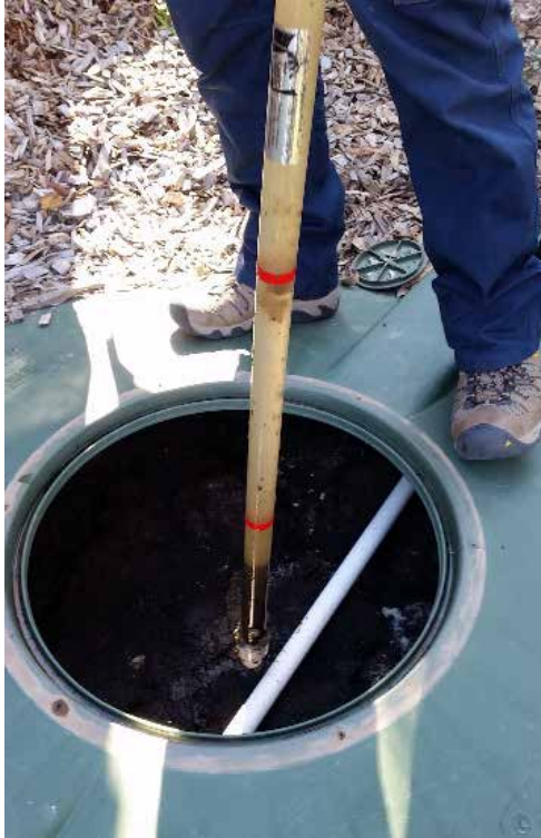
Figure 3.6 'Sludge Depth Indicator' (Source: Centre for Environmental Training, 2019)
