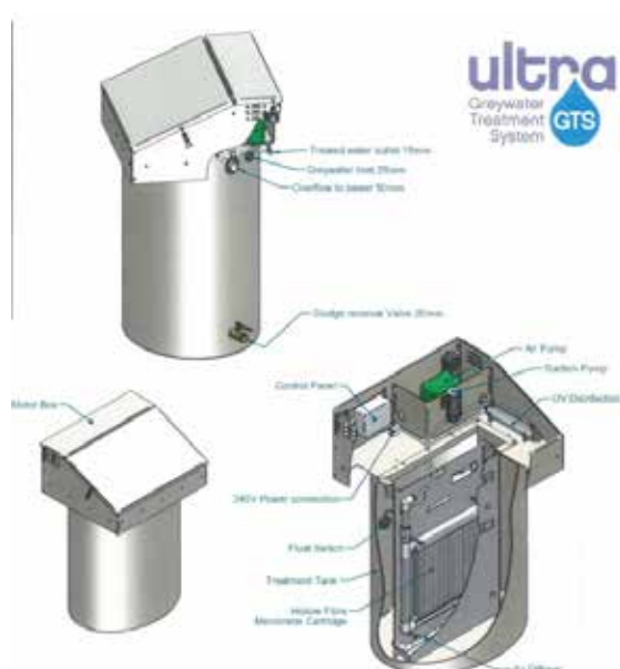
Figure 7.2 Schematic of an Ultra GTS (right) (Wastewater Australia)
